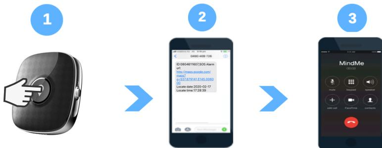
Press and hold SOS button for 7 seconds. The LED light will flash for 3 secs and an audible ring will sound. This initiates the emergency procedure
