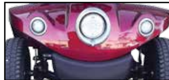
LED lighting system.
